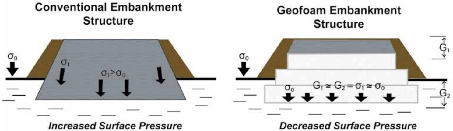
a load distribution slab to surface the geofoam,” Snow said. “For the first time, we decided to create a thicker section of lightweight concrete — about 3 feet thick, rather than the traditional 8-inch slab. This is the first time this technique has ever been used, to our knowledge. It was a cost-savings approach.”
